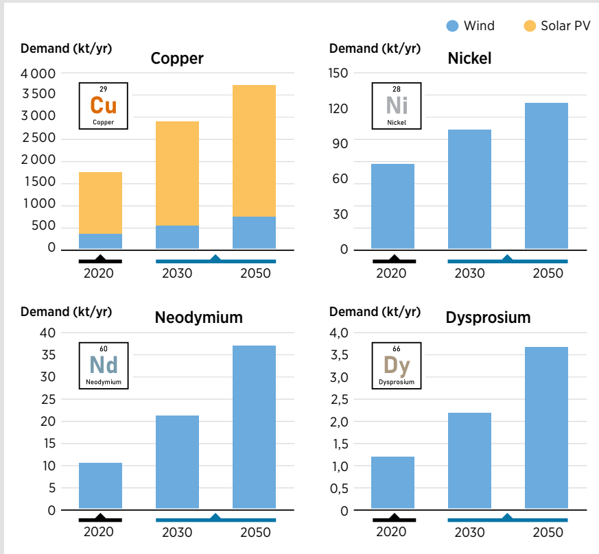
FIGURE 7.3 Projected demand for copper, nickel, neodymium and dysprosium in wind and solar photovoltaic applications under IRENA's 1.5°C Scenario
